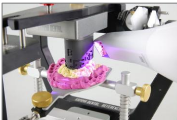
Figure 7: A bite fork scan in the articulator allows relating intraoral scans to anatomic or kinematic hinge axis.
